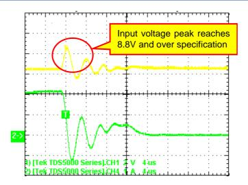
Figure 2. RT9711 power switch operated in worse condition: Vin= 6.5V, Cin= 1uF, input wire length 35cm, (Vin\_spike= 8.8V)
