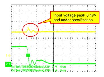
Figure 3. RT9711 power switch operated in condition: Vin= 5.5V, Cin= 1uF, input wire length 10cm, (Vin\_spike= 6.48V)
